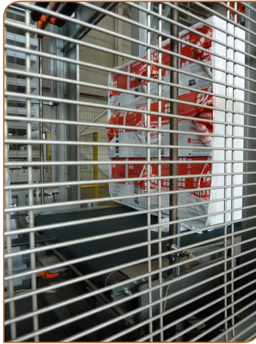
Left - Figure 8: The XPS board stacks, loosely wrapped in thermal plastic, enter the thermotunnel. Here, the plastic shrinks from the heat and the boards are then stacked ready for dispatch.
