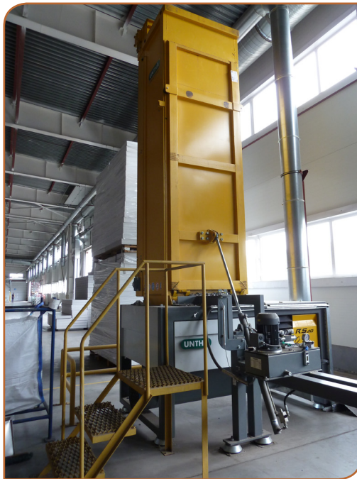
Right - Figure 9: When production changes between different board thicknesses, defective boards are manufactured more frequently. The low-quality XPS is processed in an Untha shredder for reuse.
