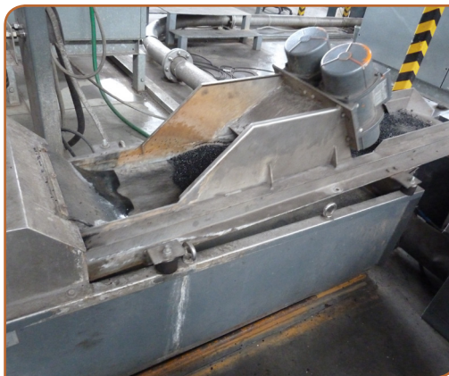
Right - Figure 10: After shredding, the waste XPS is heated to an homogeneous melt at around 190°C and is passed through tiny holes under pressure to make new GPPS granules. The resulting recycled GPPS is black instead of white and is recycled back into the XPS production process.
